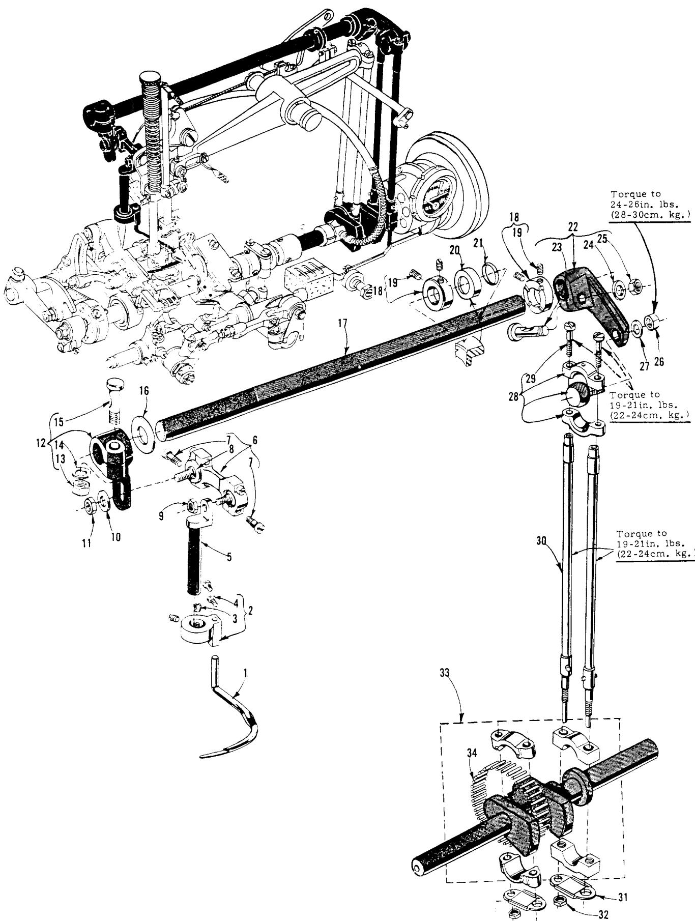
SPREADER AND SPREADER DRIVING MECHANISM
