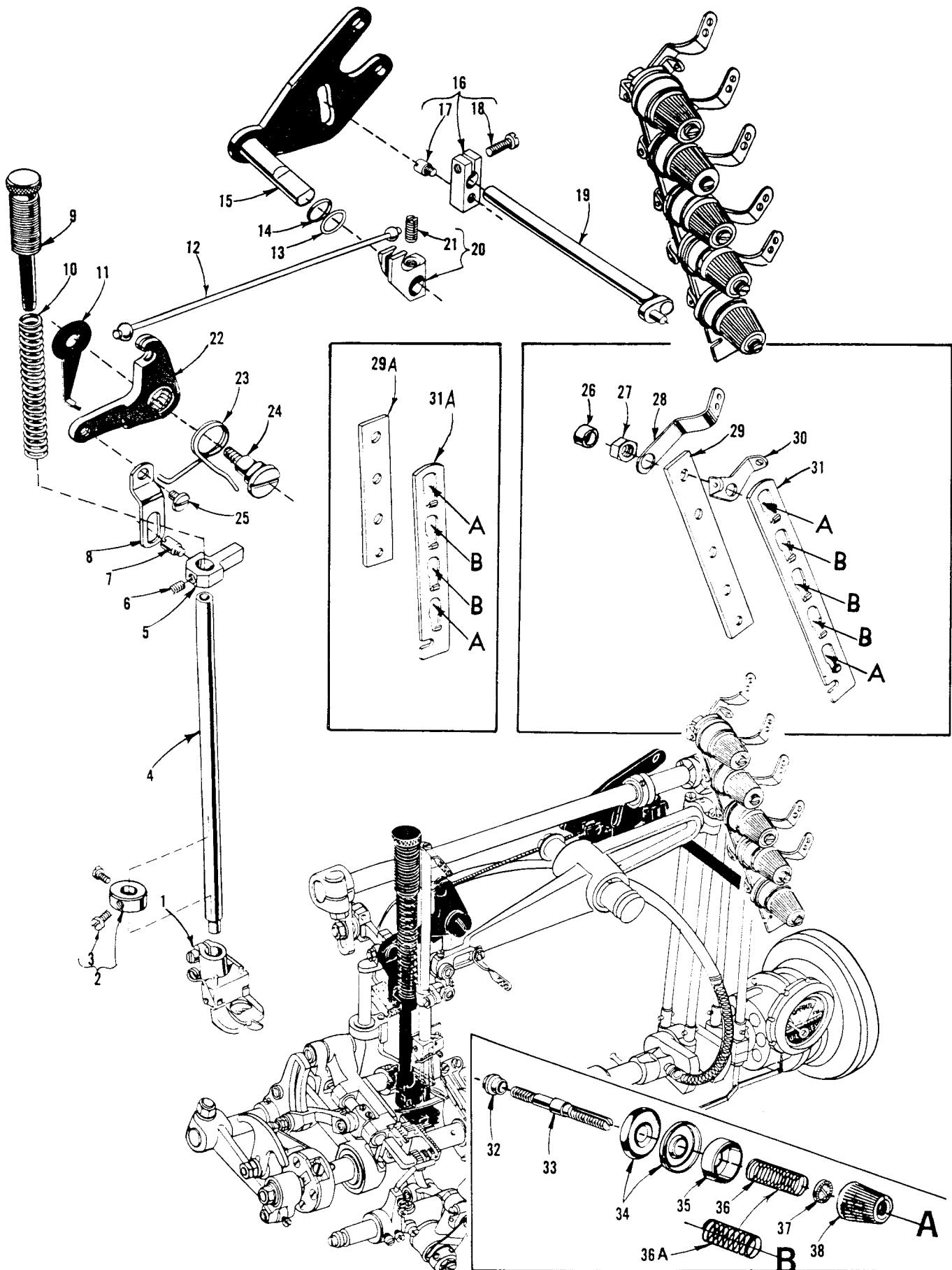
THREAD TENSION AND LIFTER LEVER PARTS
